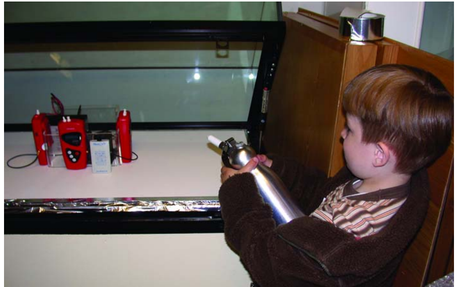
Figure 1. Sam Calver adds tracer gas to a test case using a whipped cream dispenser (without the cream). Inside the case, three PM3010 N_2O gas detectors are tested together
