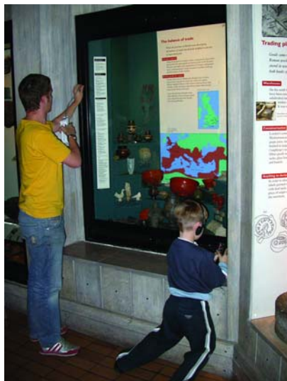
Figure 8. Andy Holbrook uses the D-TEK select and Sam Calver uses the Ultratone 100 leak detectors as part of a research project at the Museum of London. The case is deliberately vented (6 ac/d); sealing the vents only reduced the AER to 4 ac/d, suggesting most of the air was entering not through the filtered vents but elsewhere. Leaks were found along all door seams and especially around lock positions
