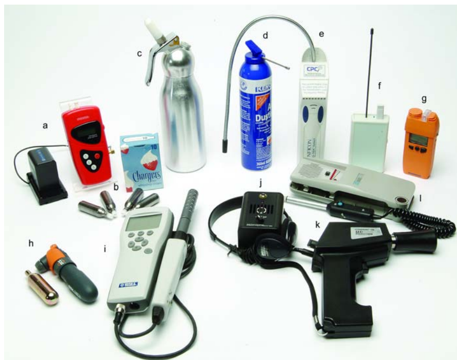
Figure 4. Selection of gas detectors, gas delivery devices and leak detectors. Top left to bottom right: (a) Medigas PM3010 N 2 O detector with additional battery; (b) N 2 O chargers 'whippets'; (c) aerosol cream whipper; (d) pressurized 'air duster' – source of halocarbon RJ 134a for leak detection; (e) D-Tek detect IR halogen leak detector; (f) Hanwell Radiotelemetry RH/T sensor; (g) Crowcon Gasman II O 2 detector; (h) CO 2 cycle tyre inflator and cylinder; (i) Vaisala GM 70 and GMP222 probe, CO 2 detector; (j) UE Systems WTG-1 ultrasonic warble tone generator; (k) Ultraprobe ultrasonic leak detector; (l) Tif 5600 halogen leak detector
