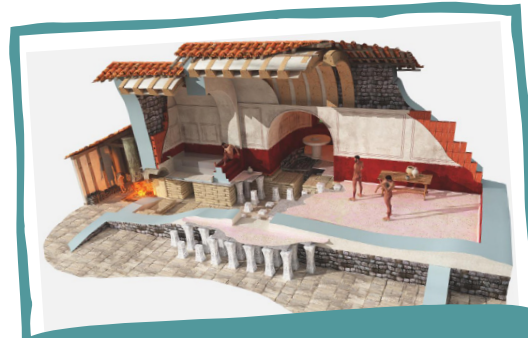
A reconstruction of the bathhouse at Chesters Roman Fort showing the hypocaust system that provided underfloor heating. This was also used in buildings such as the praetorium where the Tribune lived.
