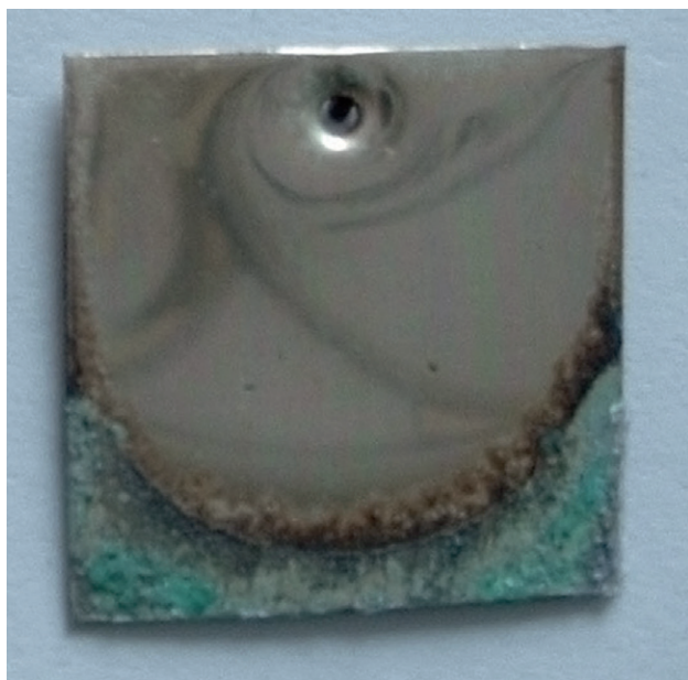
Figure 7: Example of green corrosion on high RH aged coupon
