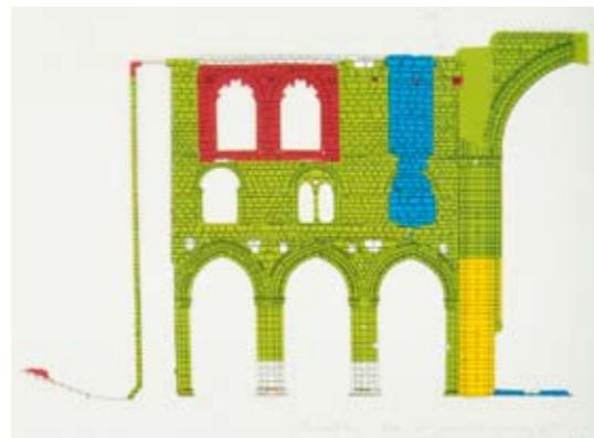
Fig. 48: The north transept arcade elevation. One of the detailed record drawings produced as part of the survey in 1989, showing some of the different building periods identified in the church. Key: yellow – early 12th century (Savigniac); green – mid- to late 12th century; blue – early 15th century; red – late 15th century; white – early 20th century
