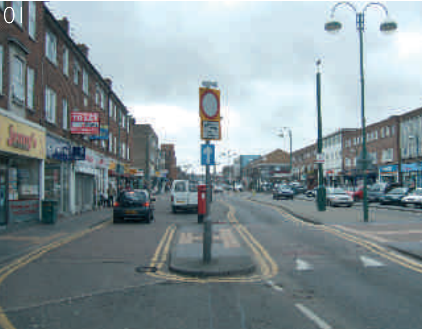
01 Borehamwood demonstrates how the excessive use of yellow lines can significantly increase the levels of visual clutter within the street
