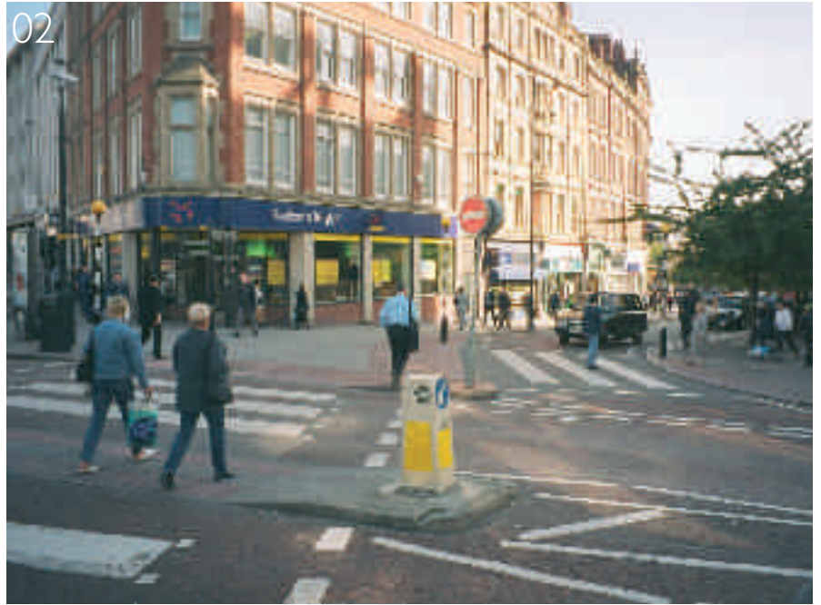
02 Zebra crossing points using excessive marking so the overall effect reduces the quality and character of the street environment
