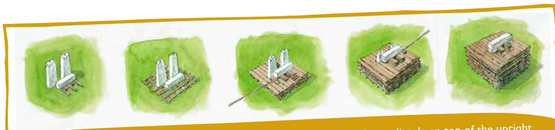
An illustration of one method that could have been used to place the heavy lintels on top of the upright stones; the stone is lifted on a growing tower of wooden platforms until the right height is reached.
