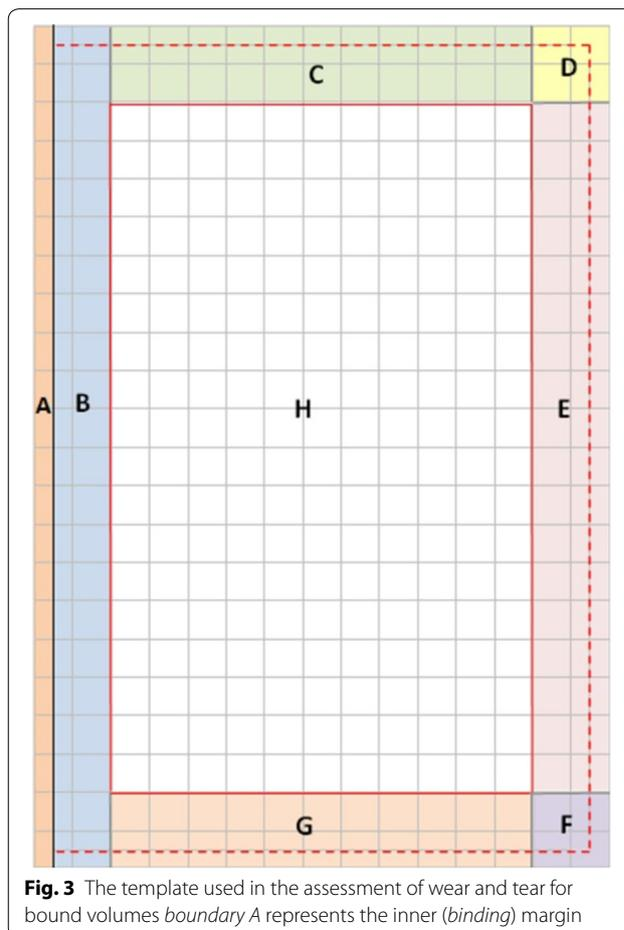
**Fig. 3** The template used in the assessment of wear and tear for bound volumes *boundary A* represents the inner (*binding*) margin
