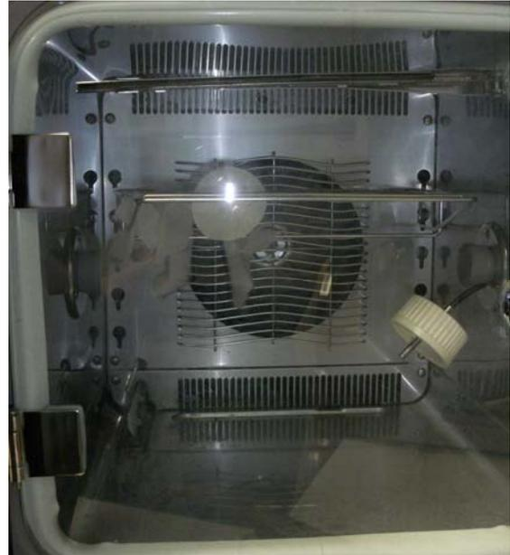
**Figure 7.5 – testing humidity levels in the RH ageing oven**
