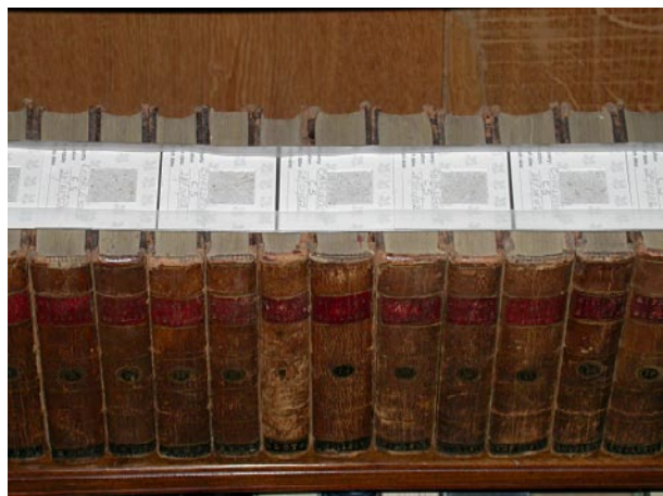
Figure 2. Close-up showing five of twelve sticky samplers attached to slide mounts and inserted in a bearer strip on a library bookshelf. Every three months one dusty sampler was removed and stored in a rigid case until the end of the three-year monitoring project.
