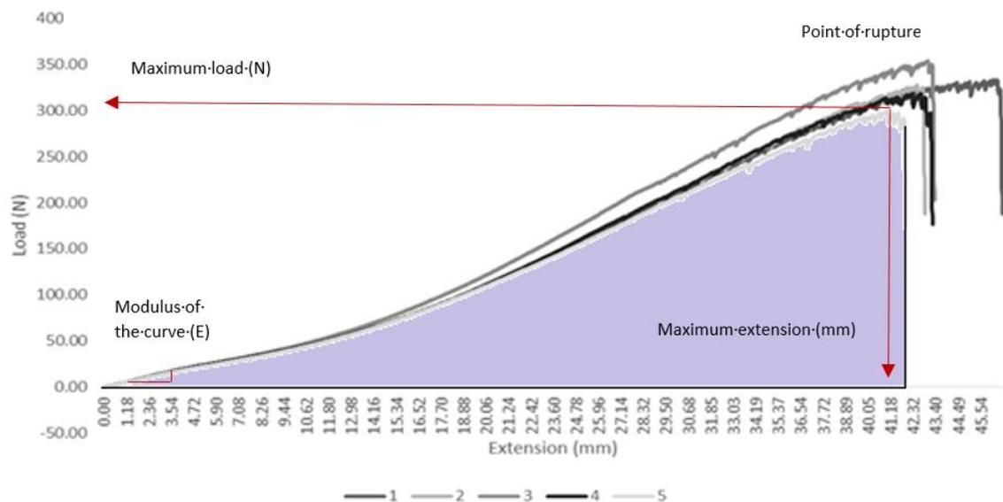
Figure 5.1- An example tensile strength curve for leather at 3mm/min extension rate detailing the key features of the curve, extension (mm) and load (N). From this the modulus of the curve (E) and the area under the curve which is equivalent to the energy required to rupture the sample (shaded area).
