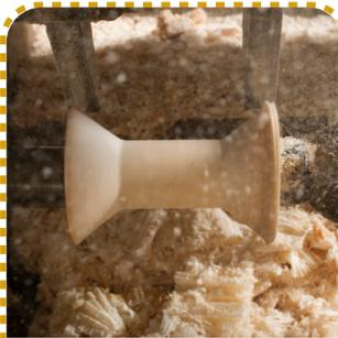
6. Once dry, the bobbin was turned on the finishing lathe to make the final shape.
