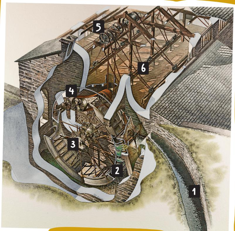
A reconstruction of the wheel pit showing the six steps it took to power the mill using the waterwheel.
