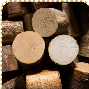
2. Using a circular saw, the poles were cut into small blocks.
