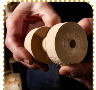
4. The block was turned into a 'rough' bobbin on a machine called the roughing lathe.
