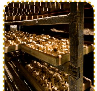
5. The rough bobbin was taken to the drying room, to completely dry out.
