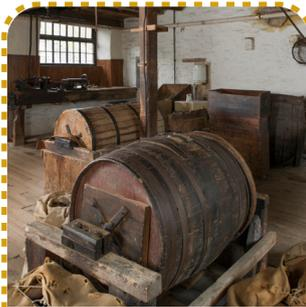
7. The finished bobbin was polished inside a tumbling barrel.
