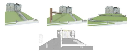
The assessors found that a spiral ramp and external escalator were unsuitable for wheelchair users, and whilst the three other options shown above provide better wheelchair access, they presented a significant issue for fire evacuation. There is no alternative escape route for lift users within the tower, and evacuation chairs are of limited use on steep, stone spiral staircases.
