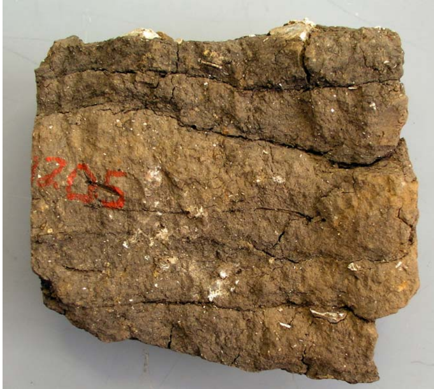
Figure 9. TS2 - Sample made up of a series of turfs from a valley gravel soil.
